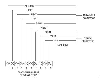
Figure 3. MPTAZ24DT, MPTAZ24DT/220 Wiring Diagram for Pan/Tilts and Lenses
